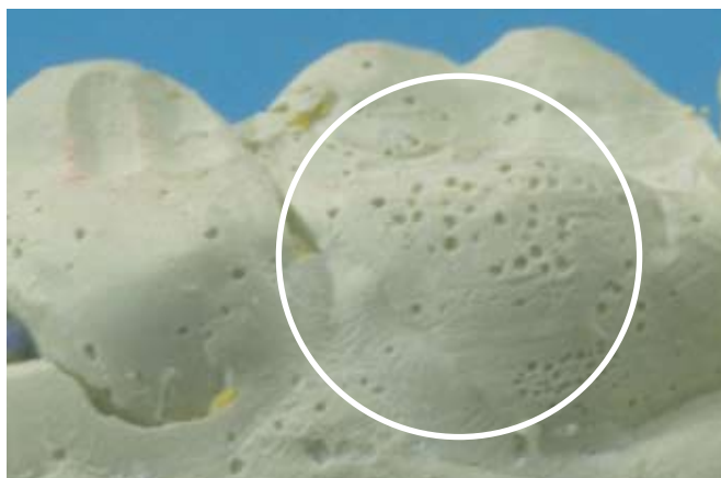
Stone Model with Hydrogen Evolution Voids
